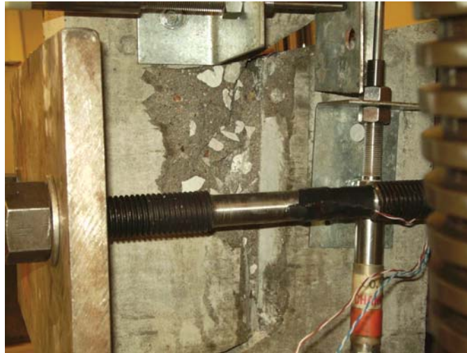
(c) Spalling of Surface on One Side, Followed by Crack Development
