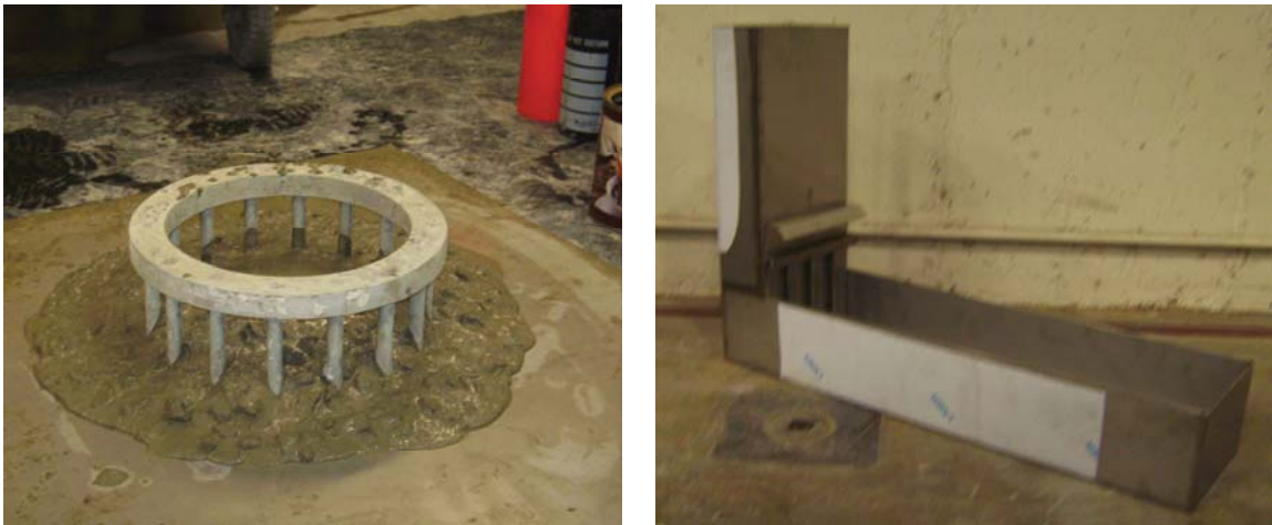
Figure 4.5 – J-ring (left) (J-ring of 22.5 inches [570 mm] pictured) and L-box (Right)
