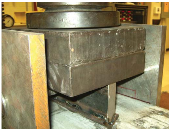
(b) Top Load Block Seated into Specimen Groove
