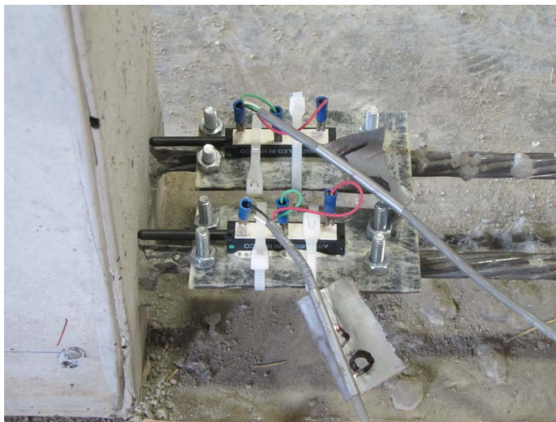
Figure 4.21 – Improved Potentiometer-FRP Assemblies with Zip Ties and Plastic Epoxy (Top) and Gorilla Glue Expanding Foam (Bottom)
