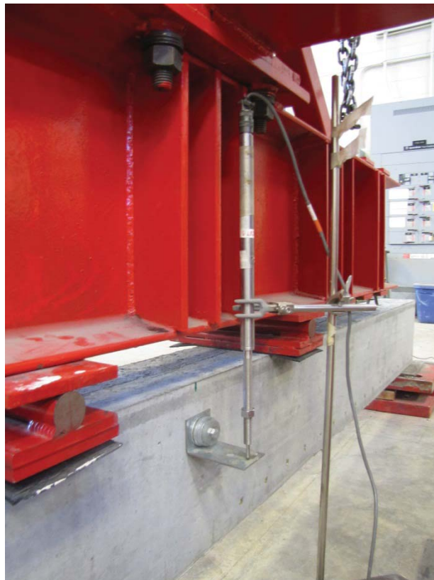
Figure 4.27 – LVDT Setup for Measuring Deflection at Midspan
