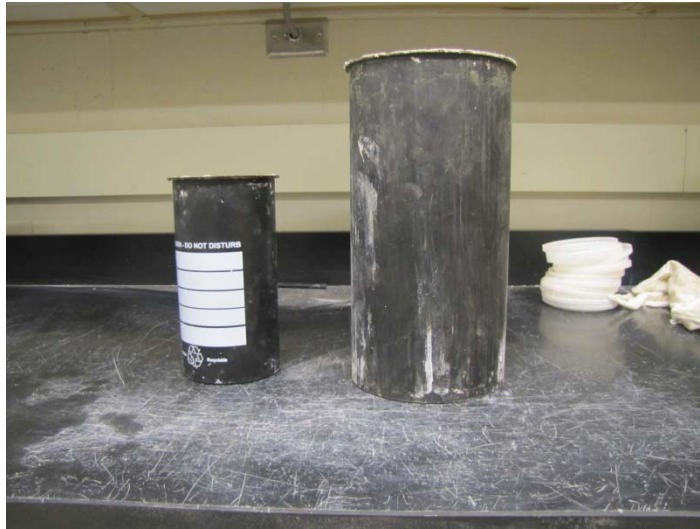
Figure 3.3 – 4 in. (102 mm) x 8 in. (203 mm) Cylinder Mold Compared to 6 in. (152 mm) x 12 in. (305 mm) Cylinder Mold
