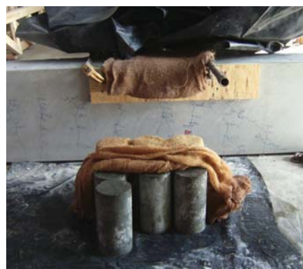
(d) "Scrub coat" and grout placed, finished (e) Cured under burlap and plastic sheeting
