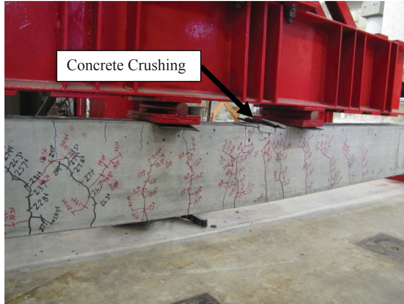
Figure F.31 – S10-2-2_73 at Failure
