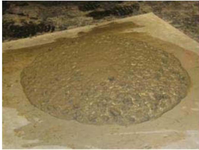
(b) Lift cone and allow SCC to flow (slump flow of 23.5 inches [595 mm] pictured)
