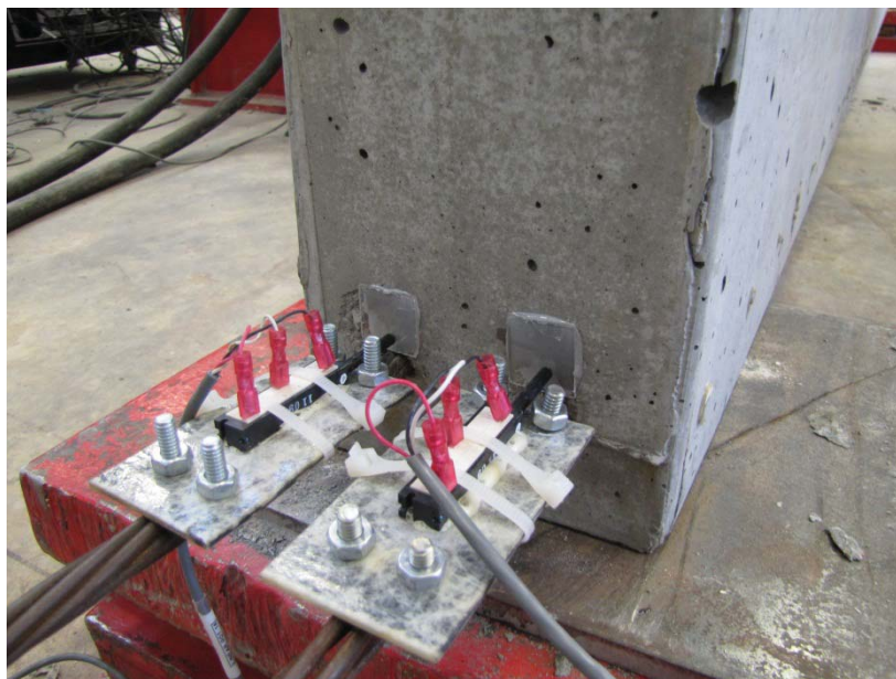
Figure 4.28 – Linear Potentiometer Setup on Four-Point Loading Tests
