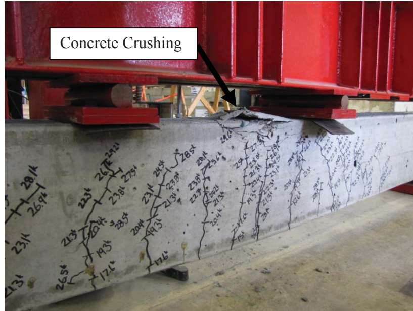
Figure F.21 – C10-2-2_58 at Failure
