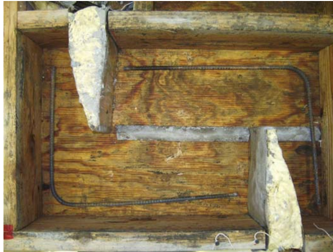
Figure 6.15 – Plan of Initial Specimen Form, Showing Cast Groove and Reinforcement Layout
