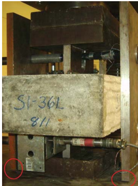
(c) Precrack Specimen Ready for Loading, Space Provided Between Apparatus and Load
