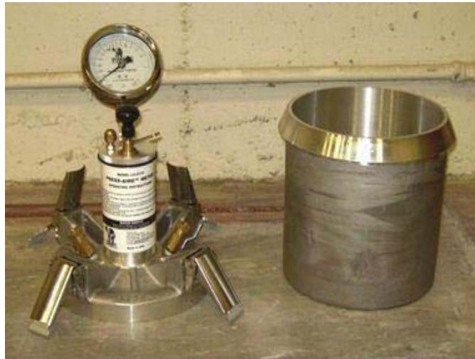
Figure 4.7 – Pressure Meter and Base Used for Unit Weight and Air Content
