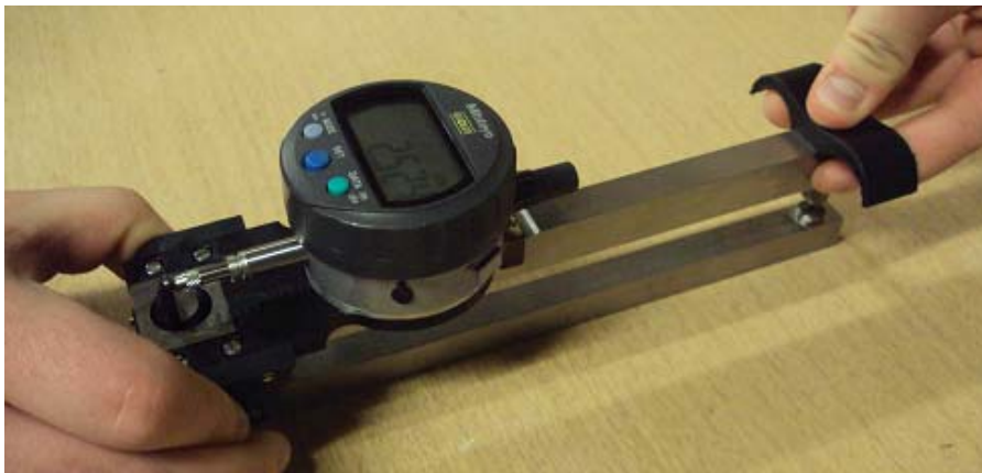
Figure 2.5 - Reading Taken on Reference Bar
