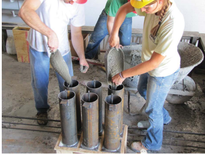
Figure 3.11 – Filling Specimens for NASP Test in Concrete
