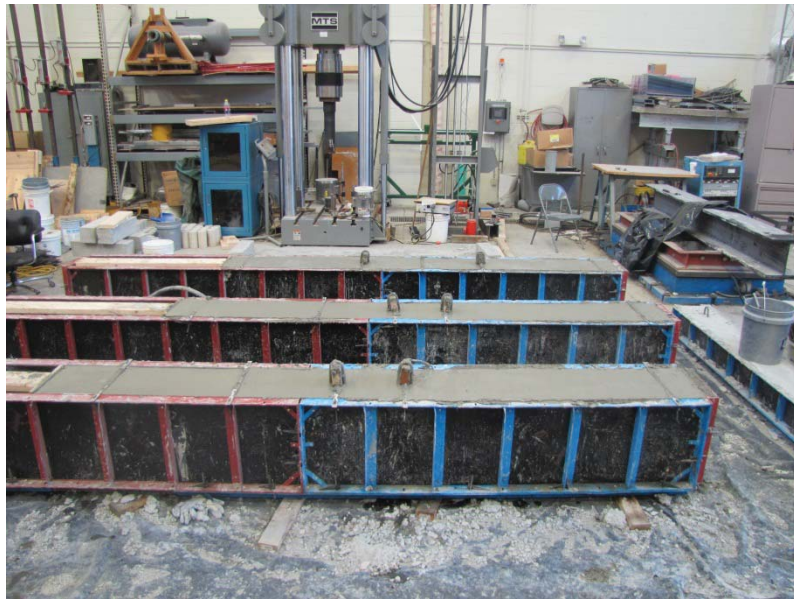
Figure 4.14 – Finished beams in forms
