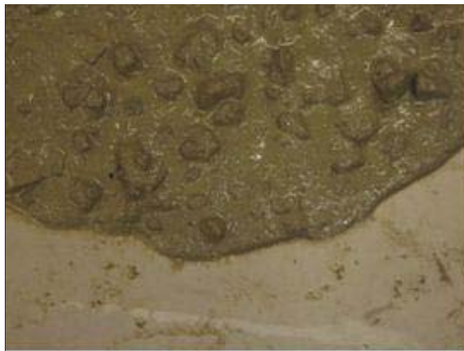
(c) Close-up for Determining VSI (VSI=1; No Mortar Halo, but Surface Sheen)
