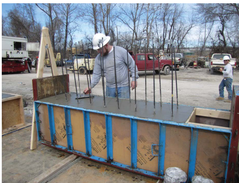
Figure 3.24 – Finished LBPT Specimen
