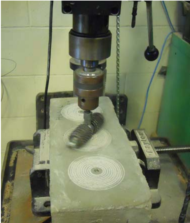
Figure 2.13 - Abrasion Resistance Test In Progress
