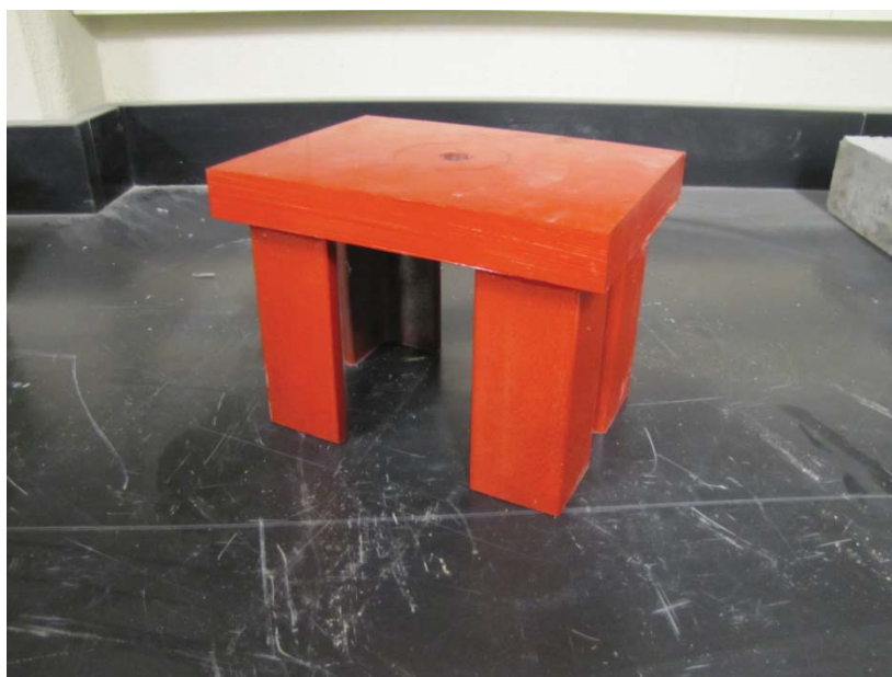
Figure 3.26 – Steel Table for LBPT
