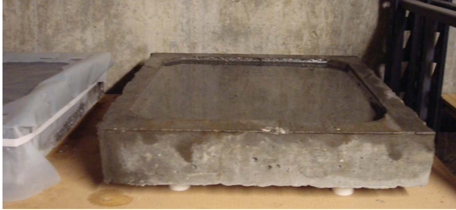
Figure 4.6 - Typical Ponding Specimen
