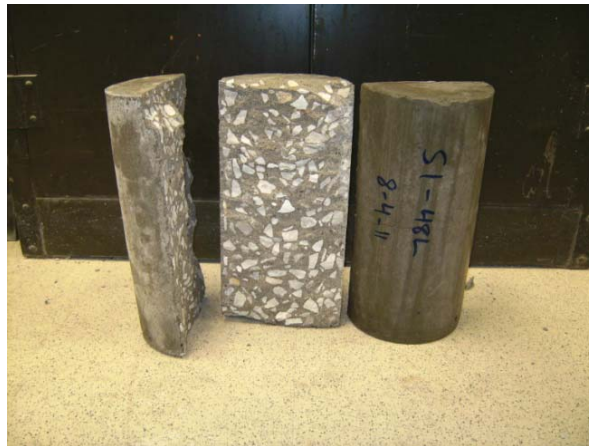
Figure 3.9 - Splitting Tensile Specimens Post-Test
