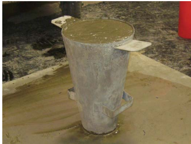
(a) Place SCC into inverted slump cone
