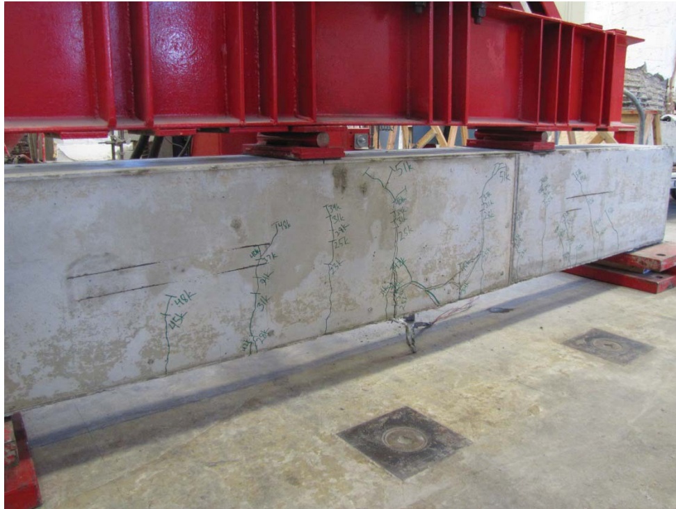
(a) Full crack pattern
