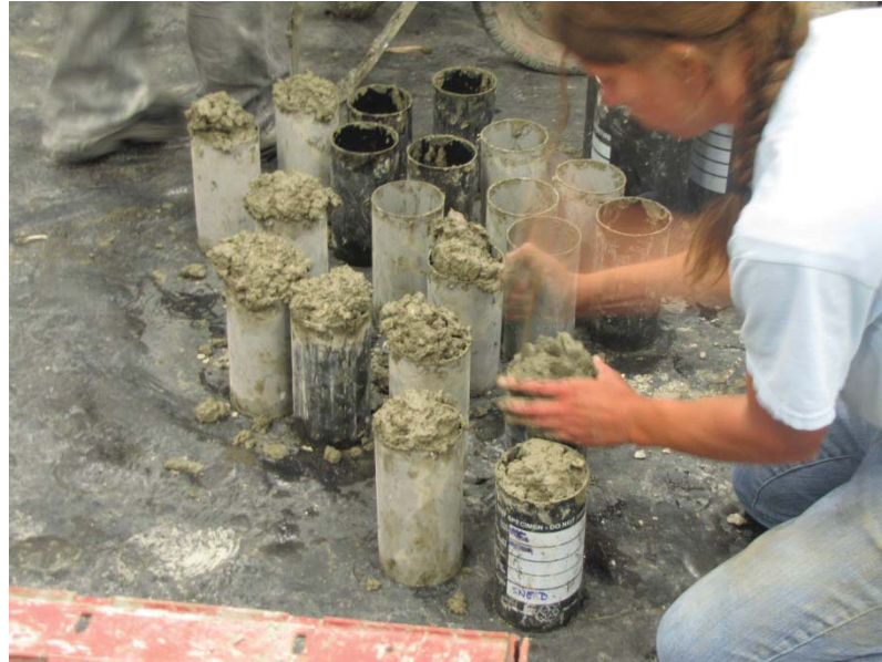
Figure 3.4 – Casting compressive strength cylinders
