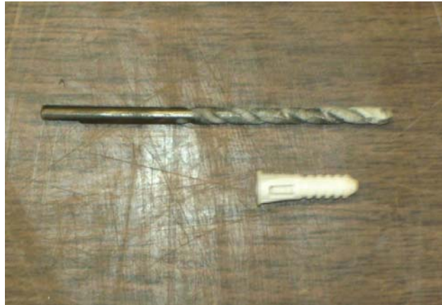
(a) Concrete Drill Bit and Plastic Anchor
