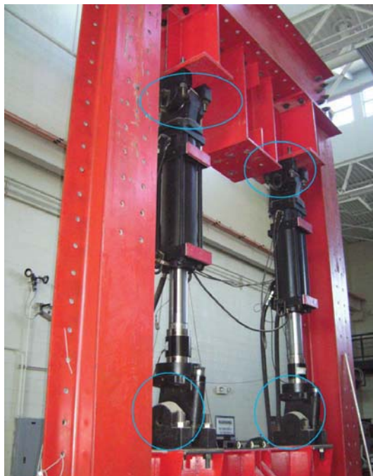
Figure 7.2 – Load Actuator used for Shear Beam Tests
