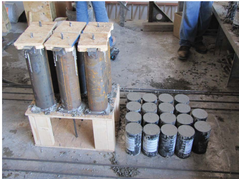
Figure 3.12 – Capped NASP in Concrete Specimens and Cylinders
