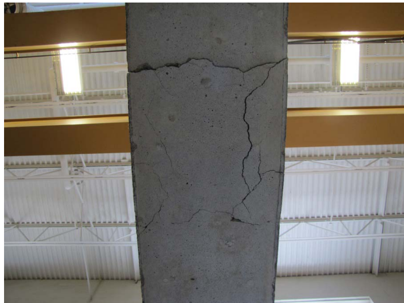
Figure 5.13 – Bottom of splice region of C6-58LBB1
