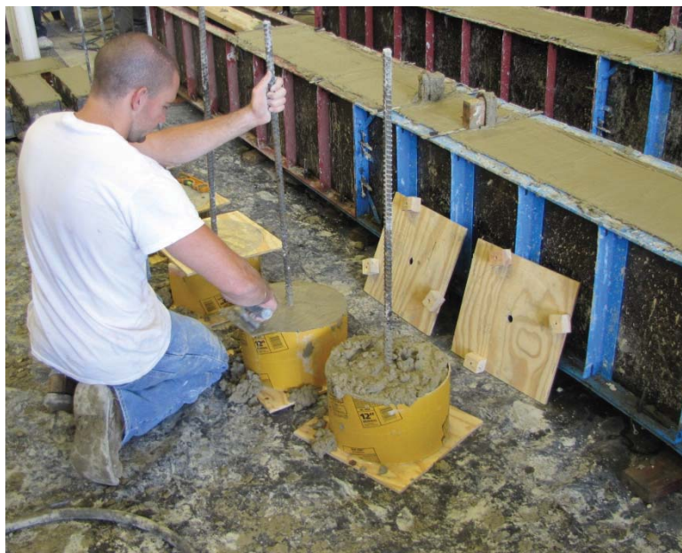
Figure 4.3 – Pull-out specimen construction
