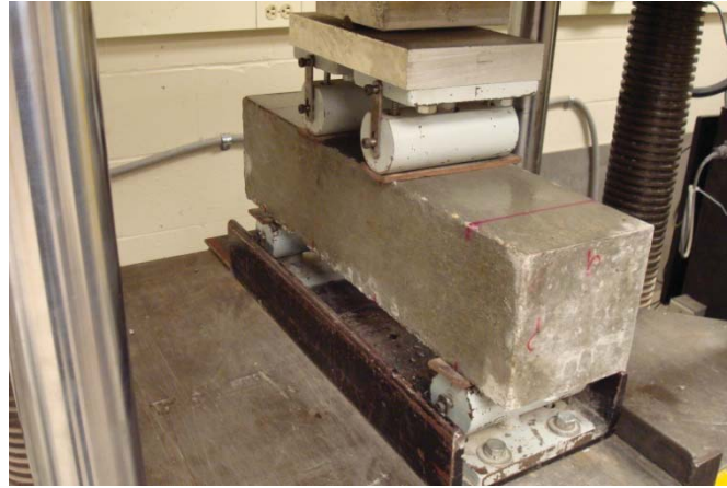
Figure 3.6 - Modulus of Rupture Testing Setup
