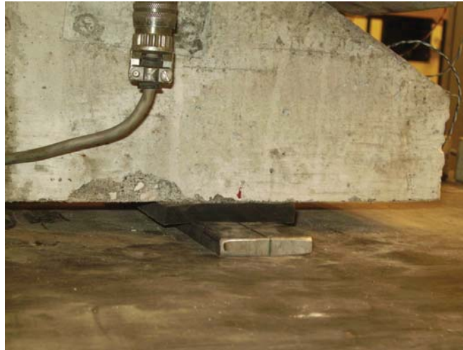
(b) Bottom Bearing Block with Neoprene Between Specimen
