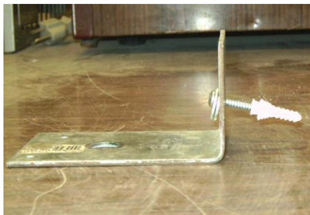
(c) Mount Installed, Anchor Expands
