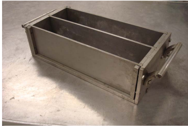
Figure 4.1 - Freezing and Thawing Specimen Molds
