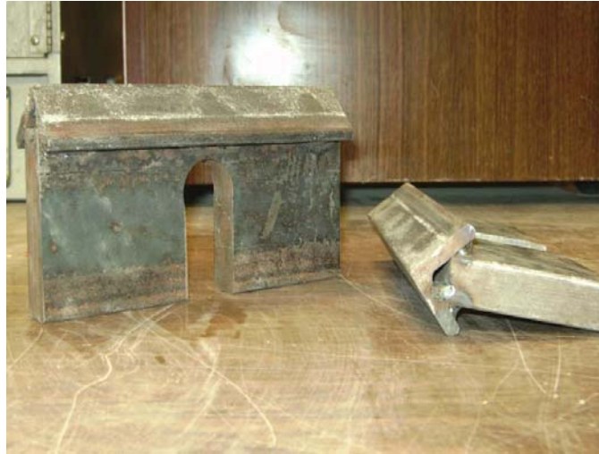
(a) Pre-crack Load Blocks
