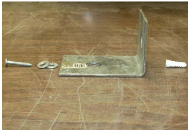
(b) Screw, Washers, Mount, and Anchor Layout
