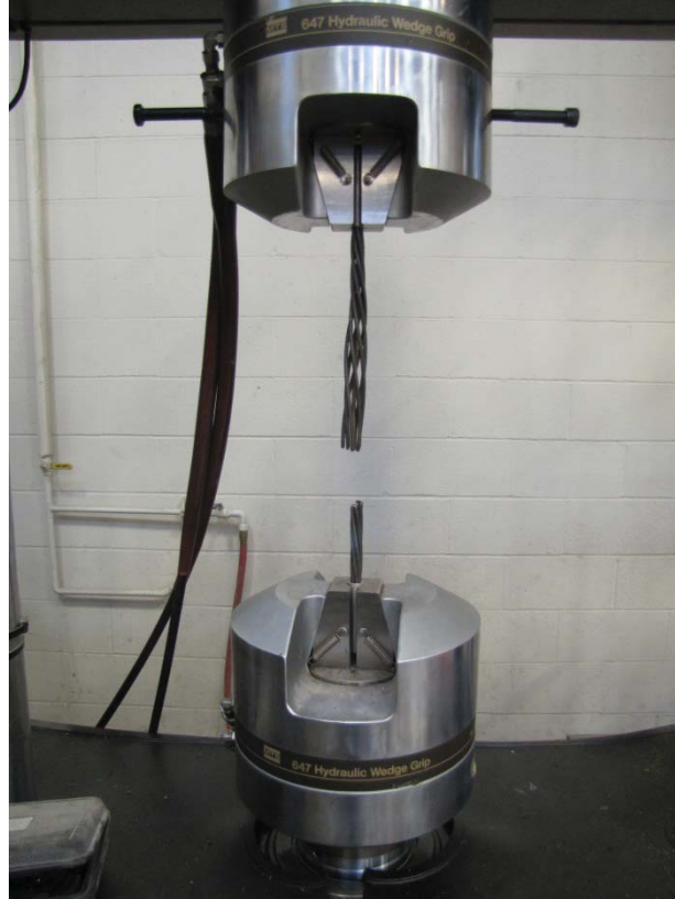
Figure 3.4 – Fractured Tension Test Specimen
